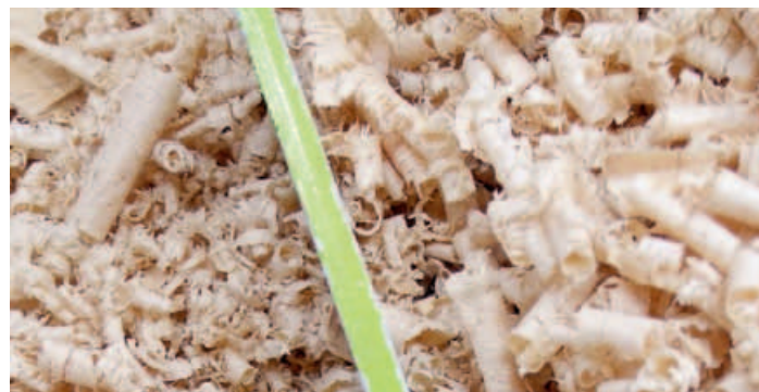
/ Interestingly, the chips of the silent power cutterblock (l.) are significantly smaller than those from the standard knife cutterblock. This has two positive effects - the chip volume is significantly reduced and the extraction functions noticeably better.
