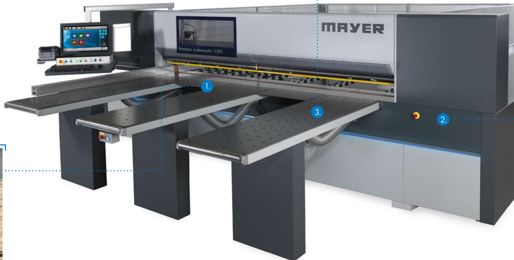
The solid air-cushion tables facilitate the gentle processing of heavy panel workpieces.
