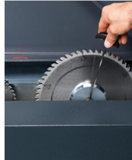
ProLock® EasyFix saw blade quick-change system guarantees shortest setup times.
