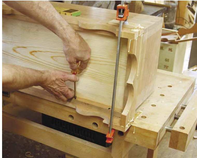
Use clamps (and protective clamping blocks) to bring the plinth together and—this is important—screw it to the case before the glue in the dovetails cures. (If you look closely, you can see the bevels around the field of the raised panel on the chest bottom. These bevels were cut freehand with a jack plane.)
