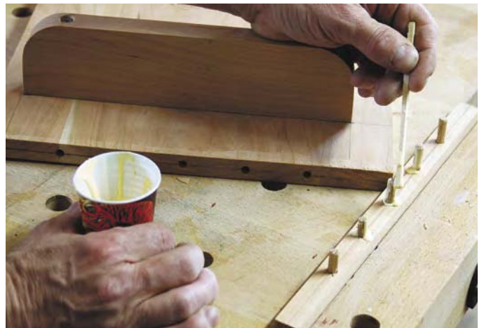
I applied glue only to the center three dowels, thinking that might allow a bit more movement across the grain of the center panel.
