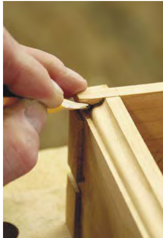
Before you glue up the plinth, mark and cut away on your band saw the surplus stock at each corner.
