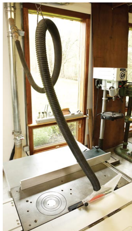
Another sucker. In addition to dust ports in the cabinet, European saws also have a dust port on the blade cover to catch debris flung from the blade.
