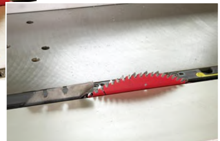
Follow the action. The riving knife behind the blade moves up and down with the blade. The knife prevents kickbacks and doesn't have to be removed for typical operations, such as cutting joints.
