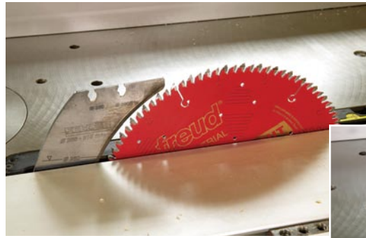
Follow the action. The riving knife behind the blade moves up and down with the blade. The knife prevents kickbacks and doesn't have to be removed for typical operations, such as cutting joints.
