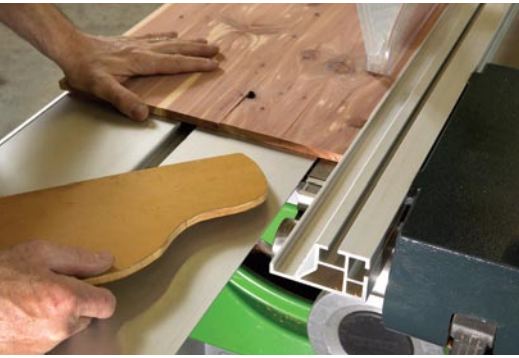
The advantage of a low fence. When ripping narrow stock, the low fence gives you lots of room to work safely.
